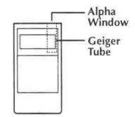
To measure as much as possible of the radioactivity of an object, place the Radalert 50 as close as you can without touching the object. The radiation level for gamma radiation from a localized source decreases according to the inverse square law. If you move to twice the distance from the object, the radiation drops by a factor of four.
