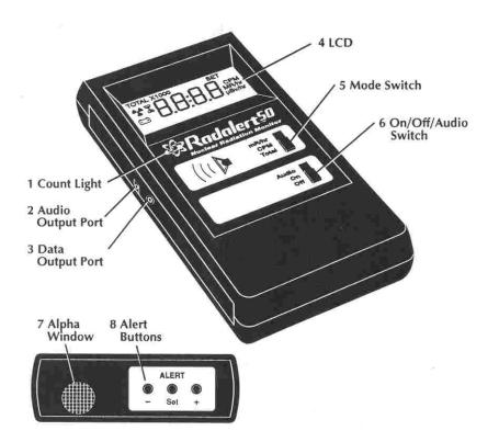
The Radalert 50 counts ionizing events and displays the results on the liquid crystal display (LCD) (4). You control which unit of measurement is shown by using the mode switch.
