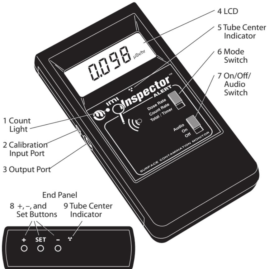
Whenever the IMI Inspector Alert is operating, the red count light (1) flashes each time a count (an ionizing event) is detected.
