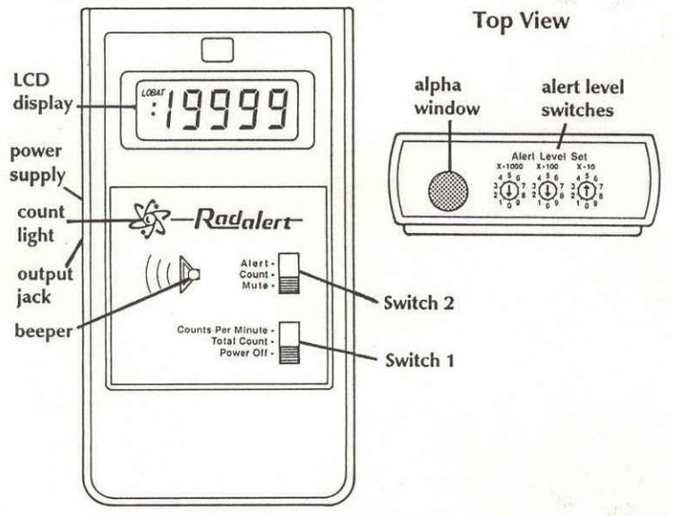
The Geiger tube in the Radalert detects ionizing events, and the electronic circuit counts these events and displays the results on the **liquid crystal display (LCD)**. You control how the counts are displayed by setting the display mode. The Radalert also contains an alert that sounds when the radiation exceeds a pre-set level that you can change for your purposes.
